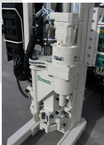
Geoprobe® GH62 Percussion Hammer & GA3000 Auger Head
